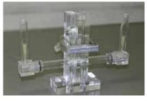
Flies perform olfactory conditioning behavior, avoiding conditioned odor that had been paired with electrical shock (left) in the teaching machine (right)
